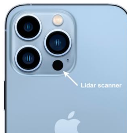
Fig 4. Camera system and lidar scanner on iPhone 13 Pro.
