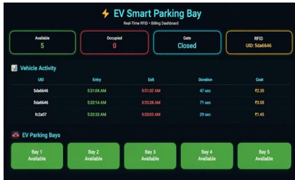
Fig. Real-Time RFID Billing and Vehicle Activity Dashboard
