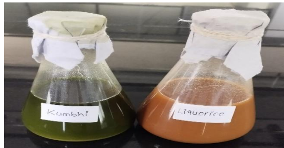
Figure 13: Extraction of Kumbhi and Liquorice by Maceration process
