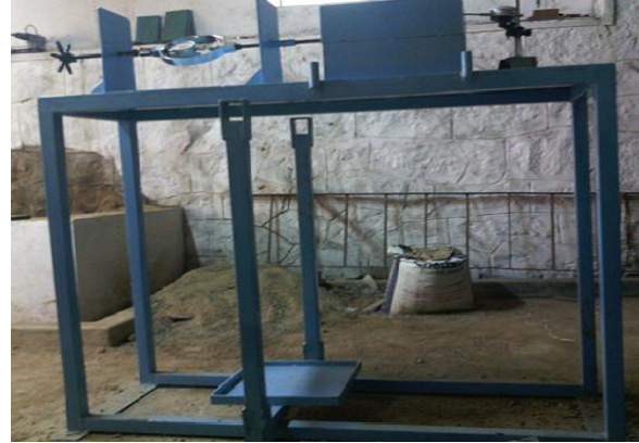
Fig.1 Large scale direct shear test set-up
