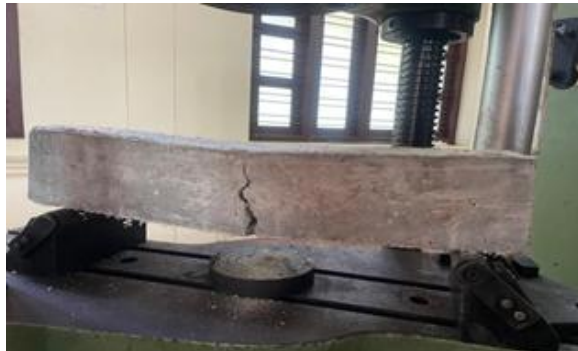
Crack pattern observation in hybrid fiber mix
