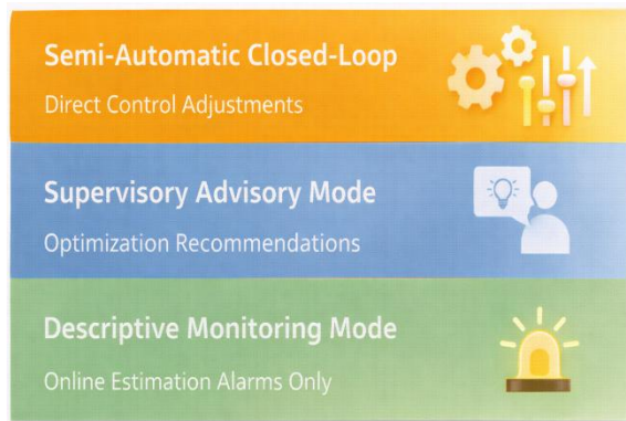
Figure 6: Three-level deployment framework for machine-learning integration in real-time paper quality control and optimization.
