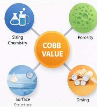
Figure 3: Key process and material variables influencing Cobb value, including sizing chemistry, porosity, drying, and surface structure.
