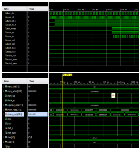
Fig.8. Fault-injected simulation waveform.
