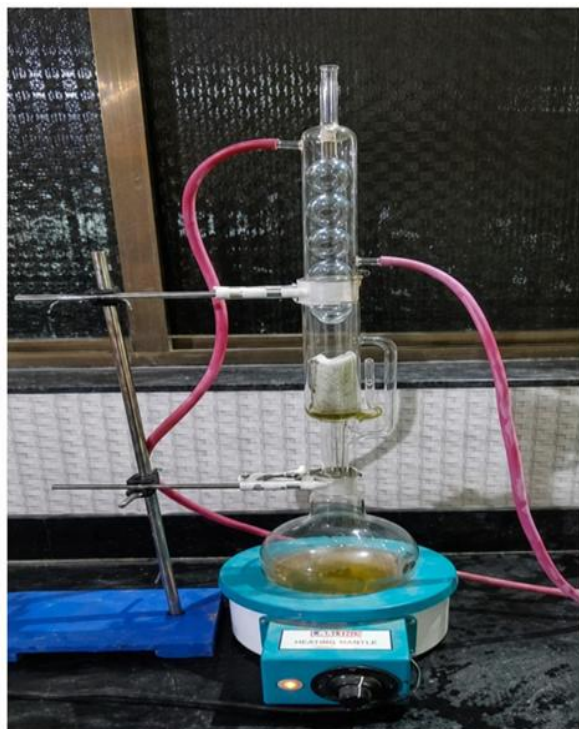
Fig. 5. Soxhlet Extraction Apparatus Used for Extraction of Moringa oleifera and Mangifera indica Leaves
