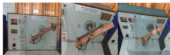
Fig 2: Different orientation of Copper Flat plate
