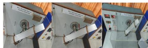
Fig 3: Different orientation of Aluminium Flat plate
