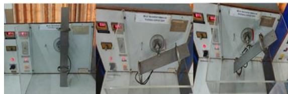
Fig 1: Different orientation of Steel Flat plate
