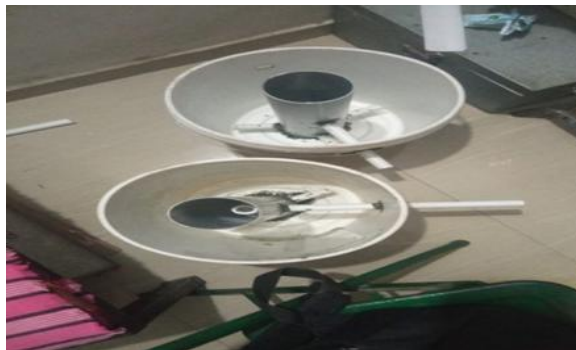
Fig. 1: Fabrication of treatment chambers showing PVC drainage and water collection arrangement.
