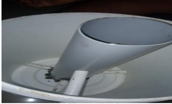
Fig. 4: Internal PVC pipe arrangement used for water collection and distribution within the filtration chamber
