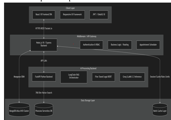
Structural Architecture Diagram of JURI AI
