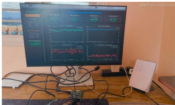
Fig. 16. Advanced EV Engineering Dashboard showing live AI model verification, BEMS telemetry, and real-time prediction charts for SOC, SOH, voltage/current, and temperature with hardware implementation using Raspberry Pi.
