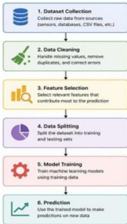
Fig. 6. Data preprocessing pipeline: raw data → cleaning → missing value handling → feature selection → normalization → train-test split.
