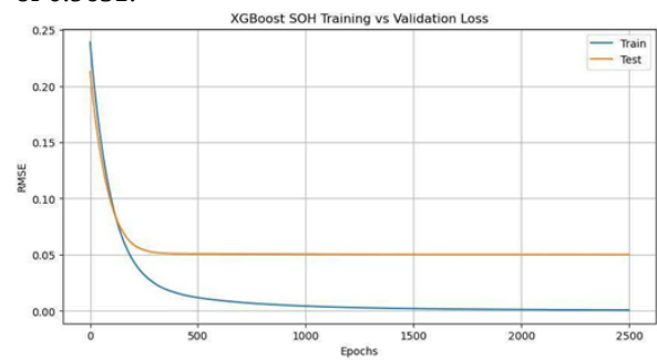
Fig. 11. XGBoost SOH training vs. validation RMSE loss over 2500 epochs.
