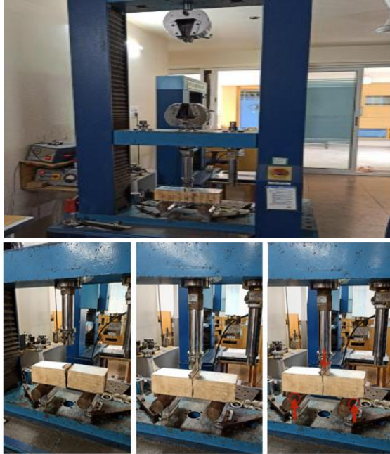
Fig. Specimen under flexural test using UTM.
