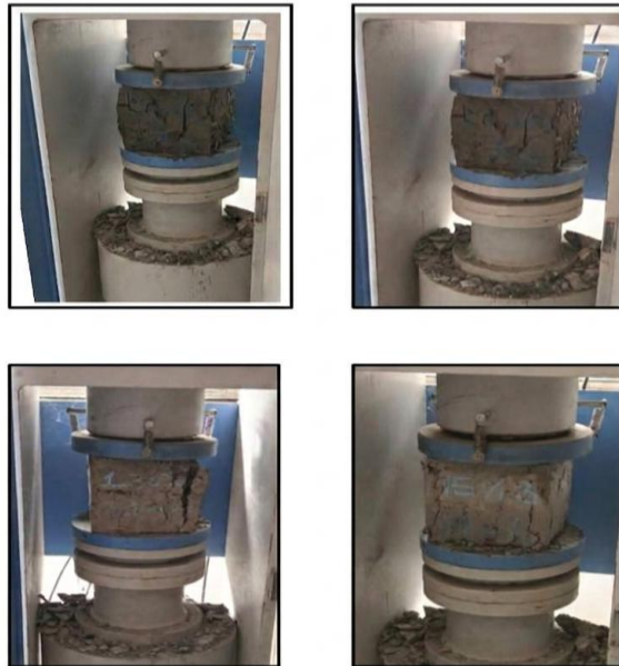
Figure 8. Failure patterns of concrete cube specimens after compression testing.
