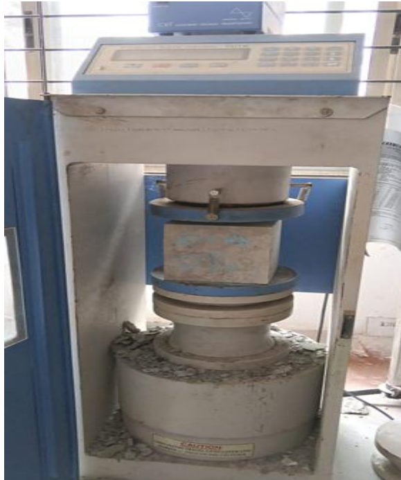
Figure 7. Compression Testing Machine (CTM) setup and testing procedure.
