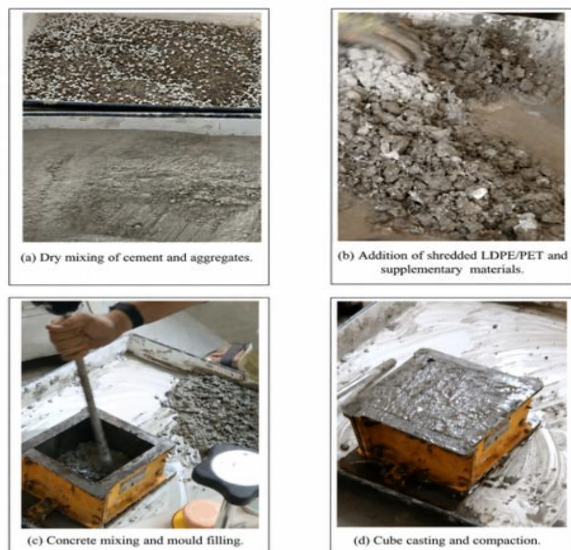
Figure 3. Concrete mixing and cube casting process.
