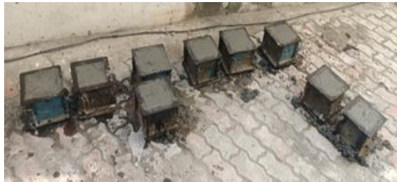
Fig 4.2 Ferrock concrete cubes
