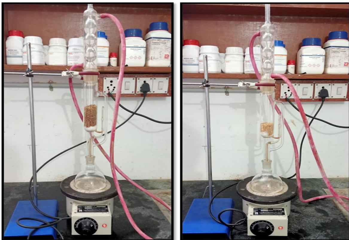
Fig 3.2(a): Aqueous extraction of pineapple and lime peels using soxhlet extractor
