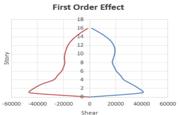
Fig. 12: First-Order Effect Storey Shear Distribution (NLTHA)
