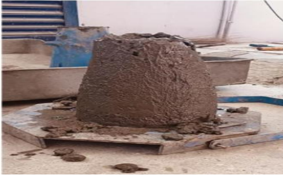
Figure 5 Slump Cone Test
