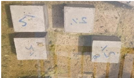
Figure 7 Curing of Conventional Cubes
