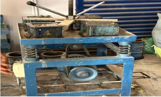
Figure 6 Compaction of Conventional concrete
