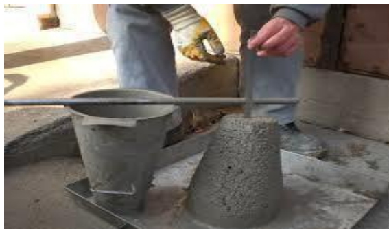
Figure: 15 Slump cone test
