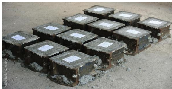
Figure: 18 Casting of Concrete
