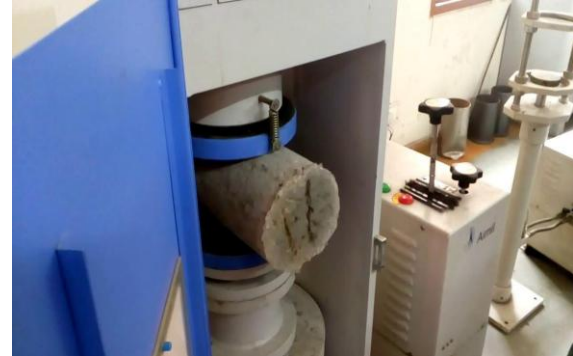
Figure: 21 Split Tensile Test
