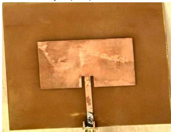
Fig. 4 [Fabricated Antenna at 2.4GHz]
