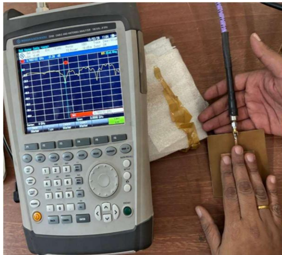
Fig. 7 [Recording resonant frequency shift]
