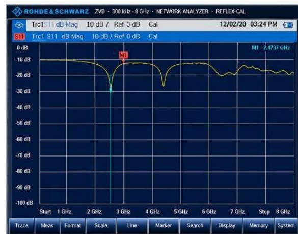
Fig. 6 [Practical result S11 parameter]
