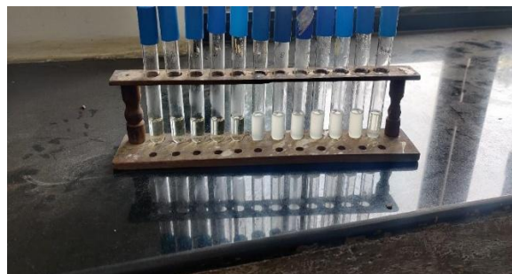
Fig 4.2: MIC of copper nanoparticles against mixed bacterial culture (concentration of CuNp's from left hand side ranging 1000, 500, 250, 125, 62.5, 31.25, 15.62, 7.81, 3.90, 1.95, 0.97 and 0 \mu\text{g/mL} respectively.)
