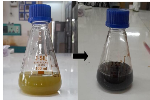
Fig. 2.1 Green synthesis of silver nanoparticles
