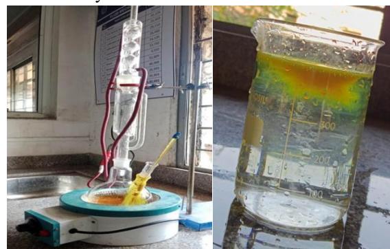
Fig: 2 Setup of extraction And Curcumin Sample
