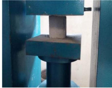
Fig7. Compression Test on Cement Mortar
