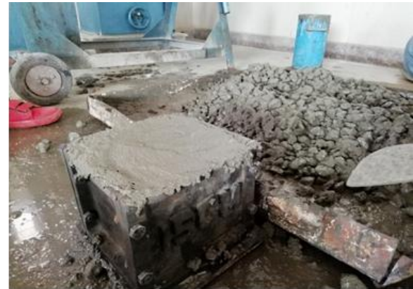
Fig 17. Casting of concrete cubes
