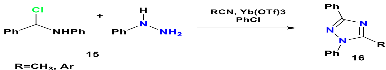
Scheme 7: Preparation of 1,2,4-triazole from phenyl hydrazine and nitriles
