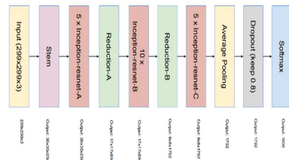
Fig. 4. Architecture of Inception ResNet V2 Model in Deep Learning.
