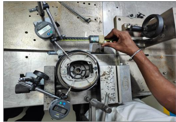
Figure 3. Test setup: the drum brake assembly mounted in the bench fixture, with two dial gauges (least count 0.001 mm) positioned against the leading and trailing brake shoes to record radial shoe expansion during cam actuation.
