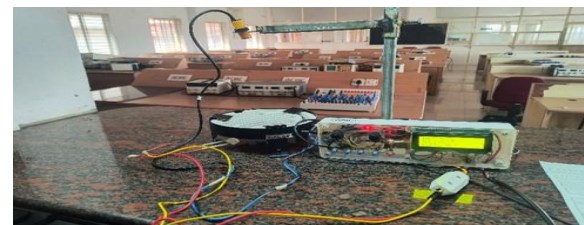
Figure 2. Front view of the final assembled Smart Electric Stove
