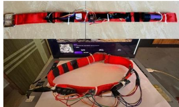
Fig. 6. IoT-Enabled Smart Pet Collar Prototype
