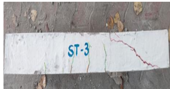
FIG 8: FAILURE OF BEAM
