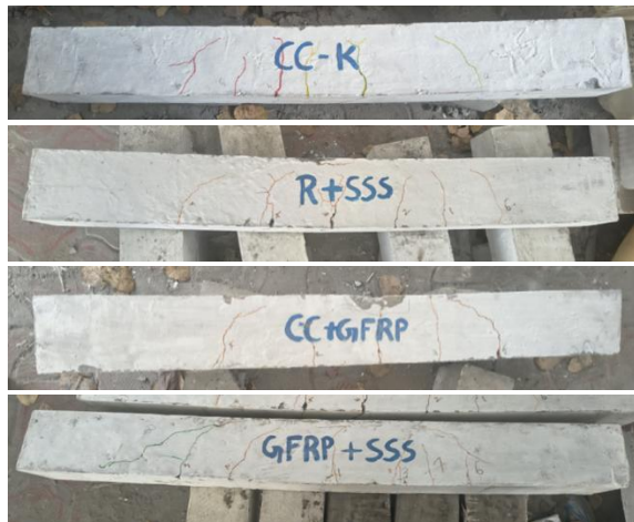
Fig 5 Crack pattern of Beams
