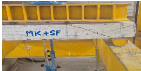
FIG 5: FAILURE OF BEAM
