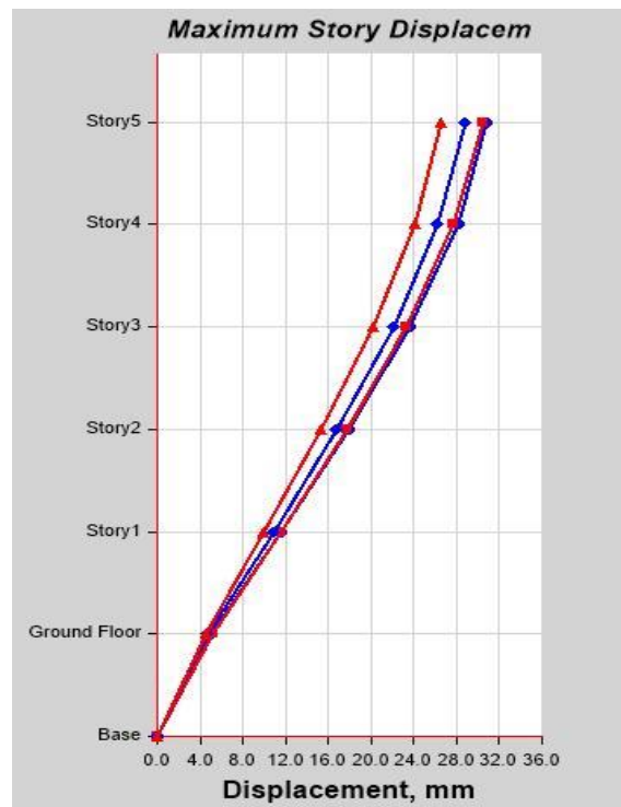
Figure 9 Storey Displacement – Normal concrete (Zone V)
