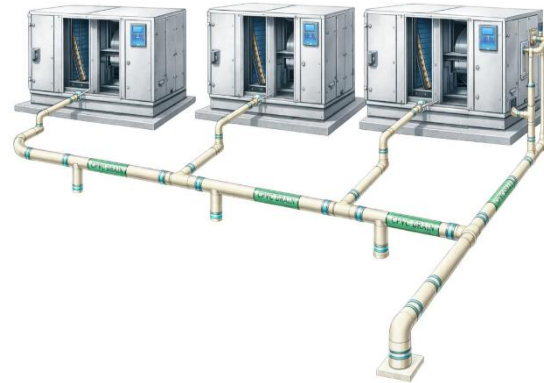
AC Condensed water collection System Image 1
