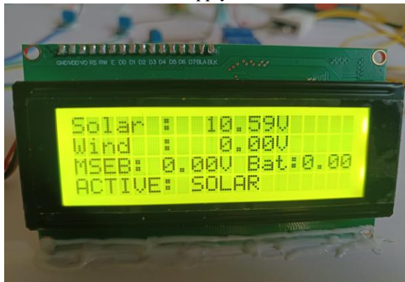
Figure 5. LCD showing Solar as the other load is not available a priority load supply
