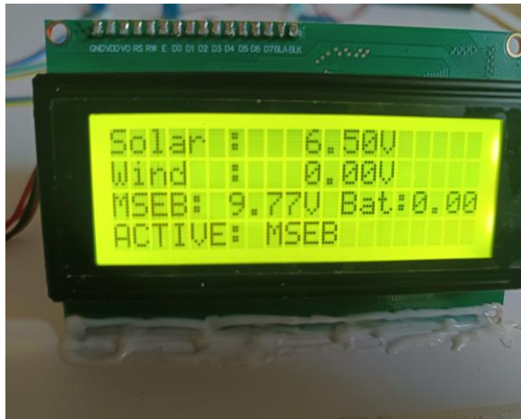
Figure 4. LCD showing MSEB as a priority load supply
