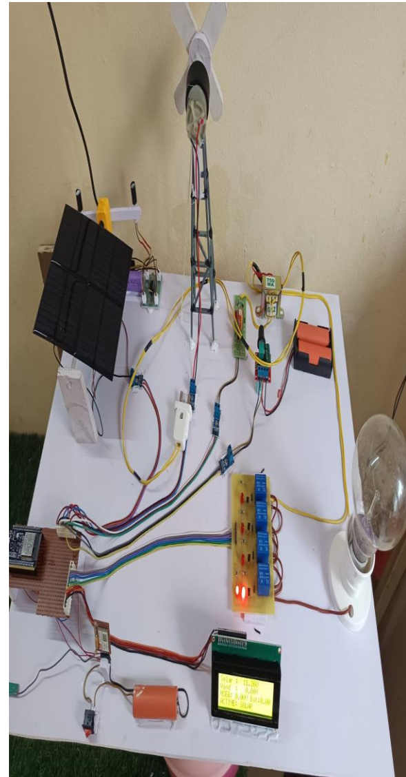
Figure 3. Prototype Hardware — Assembled IoT Smart Grid Energy Management System: ESP32 hub board, 4-channel relay module, SIM800L GSM, I²C LCD, and solar tracker
