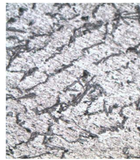
(a) As-cast LM25 (+0% wt. SiC)
