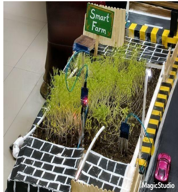
Fig. 3. Circuit prototype of the Smart Irrigation System module.
