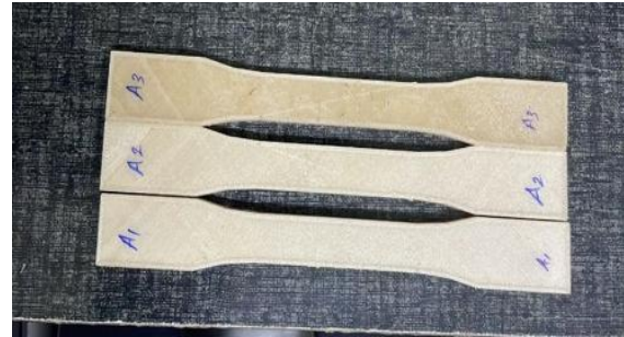
Fig. 10. FDM-fabricated tensile and flexural test specimens.
