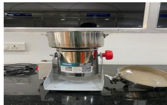
Fig. 3. Spice milling machine used to reduce the treated kenaf fibre to fine particles.
