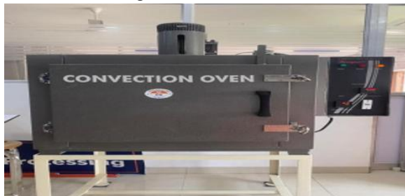
Fig. 4. Convection oven used for controlled drying of the raw materials.
