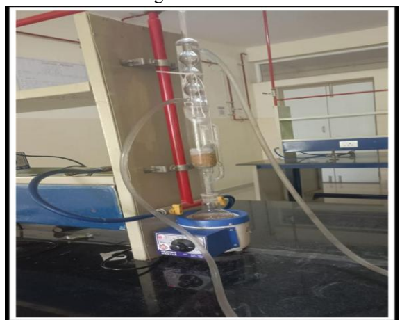
Fig. 3: Soxhlet extraction assembly used for extraction of amla seed coat
