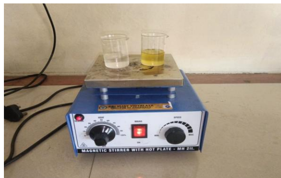
Fig. 1. Emulsification of the oil and aqueous phases on a magnetic stirrer with hot plate.
