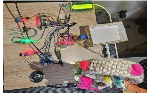
Fig. 2. Experimental Hardware Setup of IoT-Based Smart Baby Cradle
