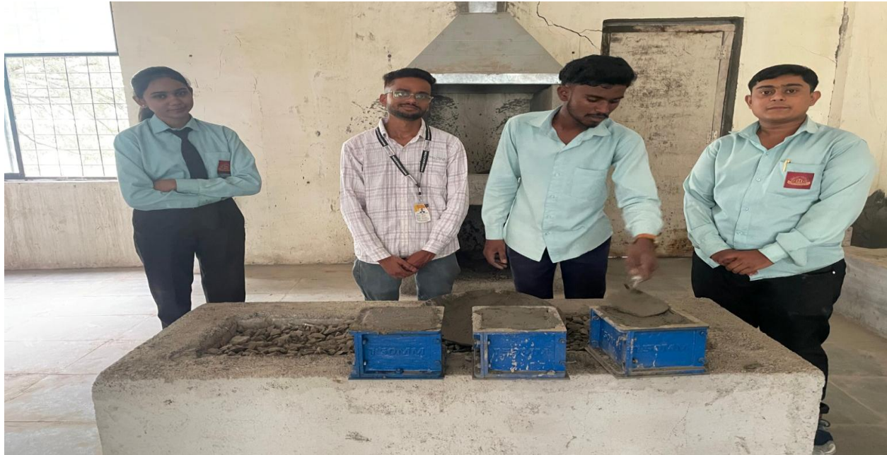
Figure 2. Preparation and casting of concrete cube specimens in the laboratory.
