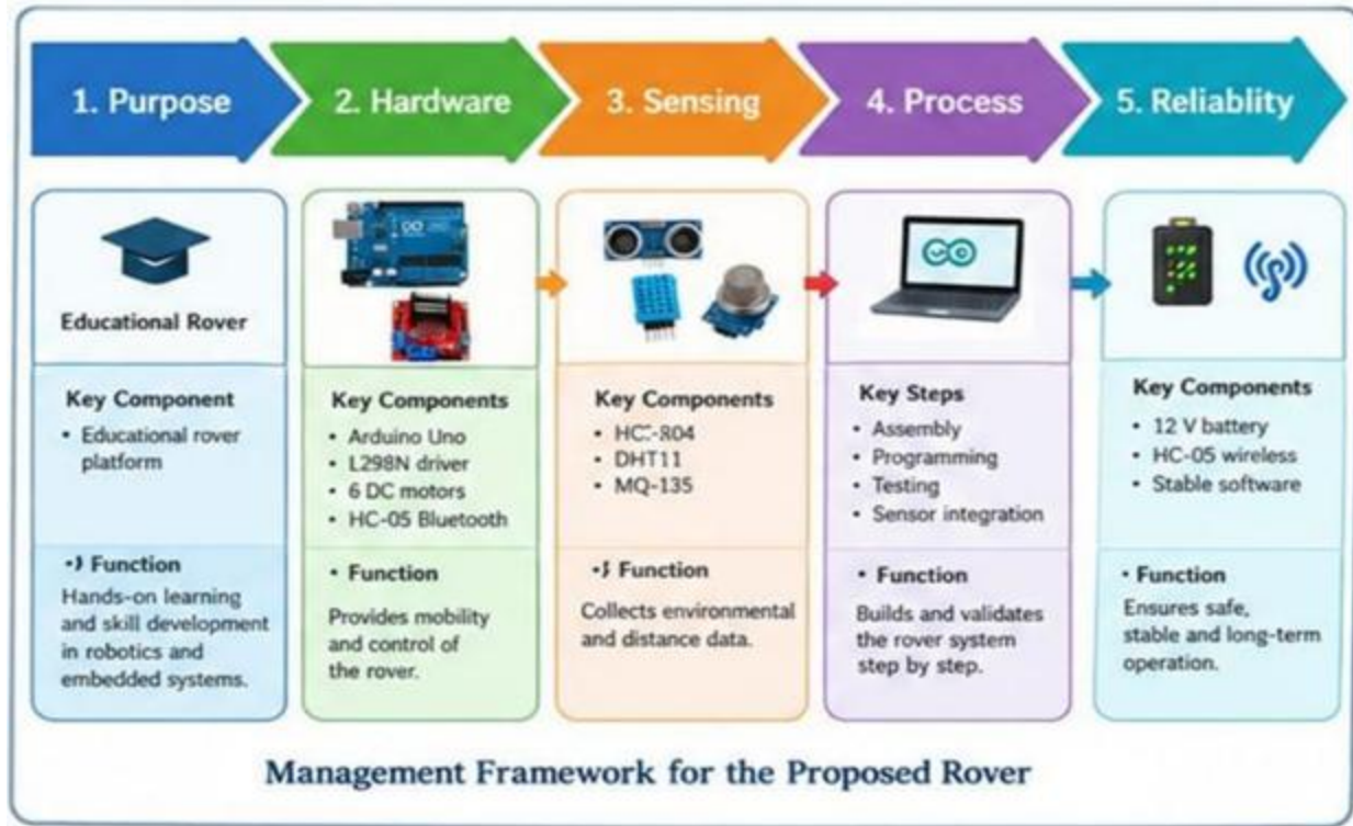
Fig. 3. Management framework diagram for the proposed rover.
