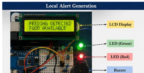
Fig. 7. Alert output using LCD, LEDs, and buzzer.
