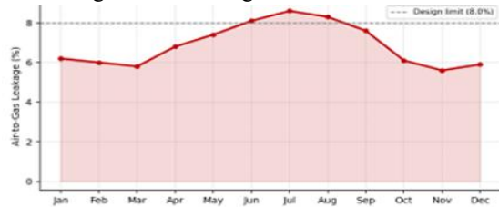
Figure 5. Monthly air-to-gas leakage trend relative to the design limit of 8.0%
