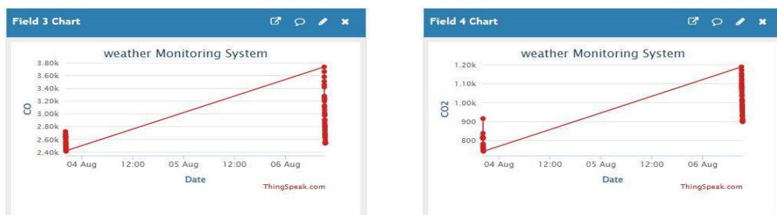
Fig. 6. ThingSpeak channel charts for CO (Field 3) and CO 2 (Field 4).
