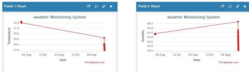
Fig. 5. ThingSpeak channel charts for temperature (Field 1) and humidity (Field 2).
