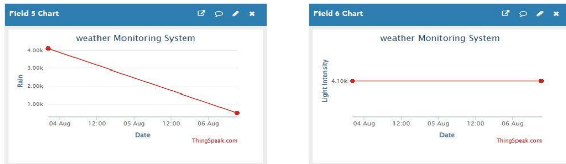
Fig. 7. ThingSpeak channel charts for the rain sensor (Field 5) and light intensity (Field 6).
