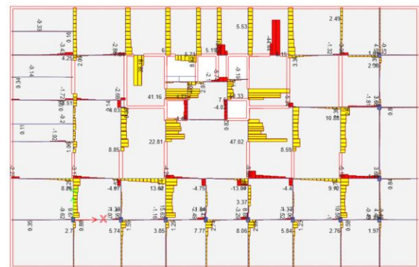
Figure 5 Forces transfer through diaphragm and collector elements for the upper bound stiffness case
