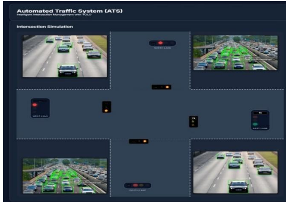
Fig. 4: Real-Time Traffic Signal and Monitoring Dashboard
