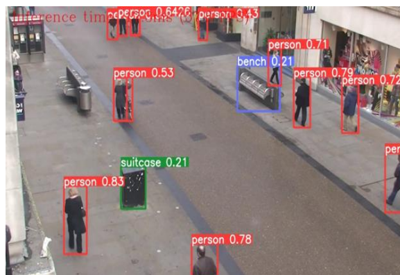
Fig. 2: Camera-Based Object Detection Using YOLOv10
